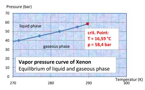
When removing (note: only from standing bottles, from above, i.e. from the gas phase!), part of the liquid xenon evaporates, but the bottle pressure remains almost unchanged - until the entire liquid part has evaporated.
