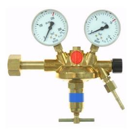
The difference between a pressure regulator and a flow regulator is easy to see on the second pressure gauge: In both systems, the first pressure gauge on the bottle side is used to check the bottle pressure and thus the filling level of the bottle. With a pressure regulator, the pressure gauge on the outlet side shows the outlet pressure set with the rotary knob at the bottom in the printed unit bar or psi.
