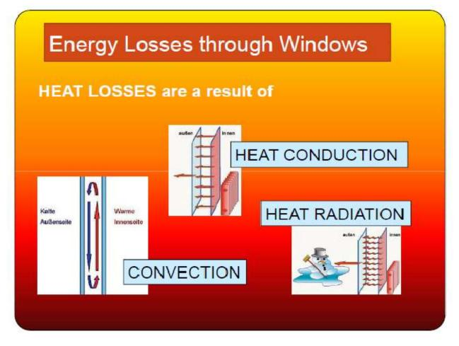
For this purpose, optimized double or multiple panes of glass have been used in Central Europe for several decades. Equipping the basic glass with coatings of low emissivity (low- $\epsilon$ ) leads to an almost complete elimination of the <u>radiation losses</u> through the glass units with the desired thermal insulation.
