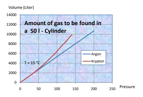
In the case of argon, this simple estimate underestimates the amount of gas actually present in the bottle by up to 7%, and in the case of krypton by almost 30%, since both gases in the bottle are gaseous at room temperature, but only approximately the above-mentioned ideal gas law  $p^* V = const.$  correspond to.
