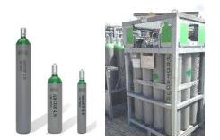
Depending on consumption, gas can be delivered in 10 I, 20 I or 50 I bottles or in bundles. The filling pressure of these pressure vessels is usually 200 bar, although there are also 300 bar bottles. This high compression makes it possible to transport large amounts of gas in a space-saving manner, even if our gas filling devices get by with a significantly lower inlet pressure.
